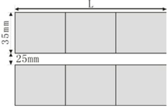
$L = (80 \times n) - 14$ <p>n: 每排报警器的个数</p> <p style="text-align: right;">单位：mm</p> |
